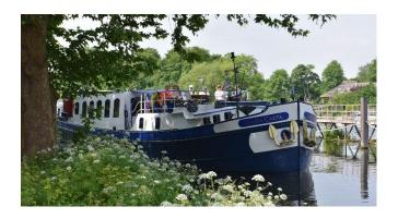
Former purpose: Ex Sand Cargo Barge operating in Holland Original year of construction: 1936 in Holland Dimensions: 117ft (35.6m) Length, 16ft 6" (5.05m) Width Year converted to a Hotel Barge: 2001 / 2002 Generators: 230-volt 48kva generator and
